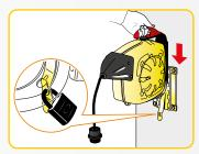
To prevent removal or theft of the cable reels it is possible to secure it with a bolt or a lock.
