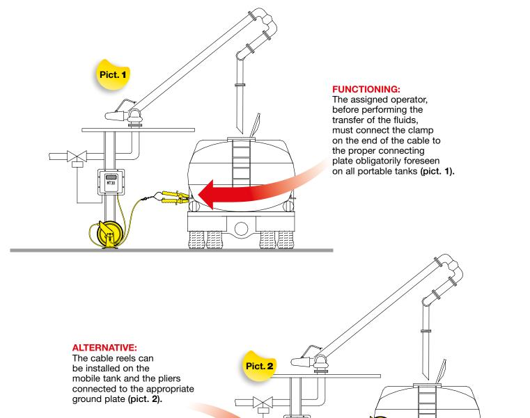
**The cable reel easily meets** the need to ground the tanks containing flammable liquids during the operations of transfer in order to avoid the accumulation of dangerous electrostatic charges.
